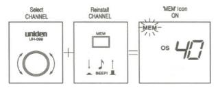
When finished, rotate the **CHANNEL SELECTOR** dial and notice that the **MEM** icon is indicating which channels are programmed and which have been removed.
